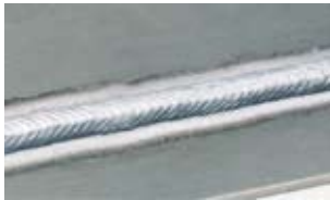
用Pulse-On-Pulse™工艺焊接3mm厚的铝
